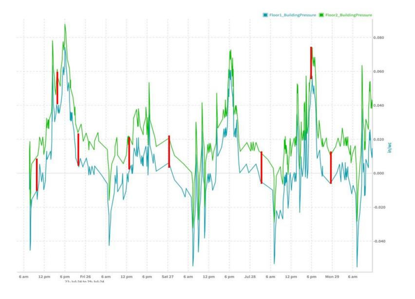
Extensive cycling of air pressure on floors during typical day
